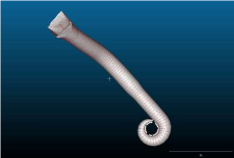
Figure 7. Model of a penstock generated from multibeam sonar data.
