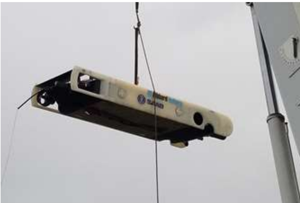
Figure 2. AUV (Saab Sabertooth. Double hull) can be equipped with 3D sonar, remote cameras, LED lights, range of more than 20 km.
