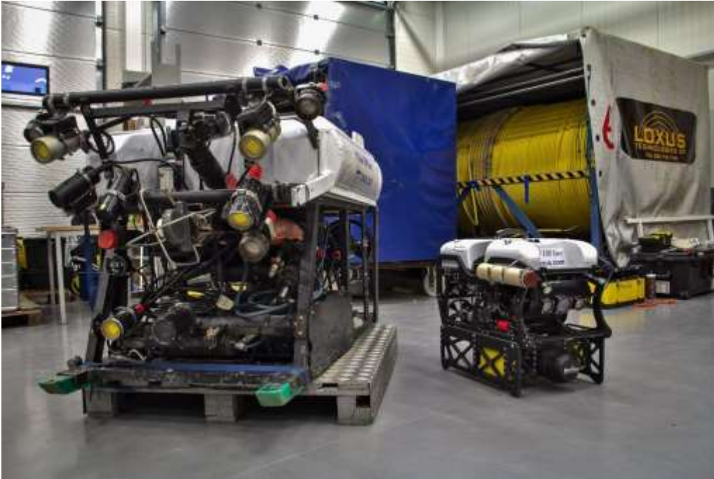
Figure 1. Several types of ROV. Loxus Explorer (left) 3D sonar, remote cameras, LED lights, range up to 7km; SEAMOR Marine Chinook - multibeam sonar, cameras, lighting, range up to 2000m.
