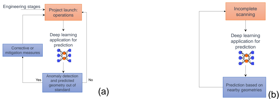
Figure 2. Application scheme of a prediction algorithm. (a) Explanatory diagram of a prediction algorithm applied during the horizontal advance per blast cycle (b) Explanatory diagram of an incomplete scanning estimation.
